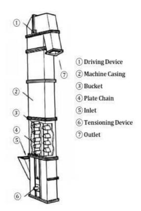
• **Base**: it is composed of machine base shell, bottom wheel, tensioning device, feed hopper and induction devices.
