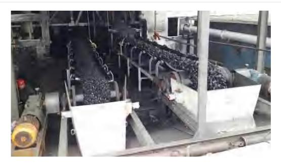
Coal preparation plant is a coal processing plant that include a series of processes: raw coal screening, crushing, coal washing, separation, clean coal dewatering and slime recycling. Which can separate coal from impurities, remove mineral impurities from raw coal and divide it into different specifications of products.
